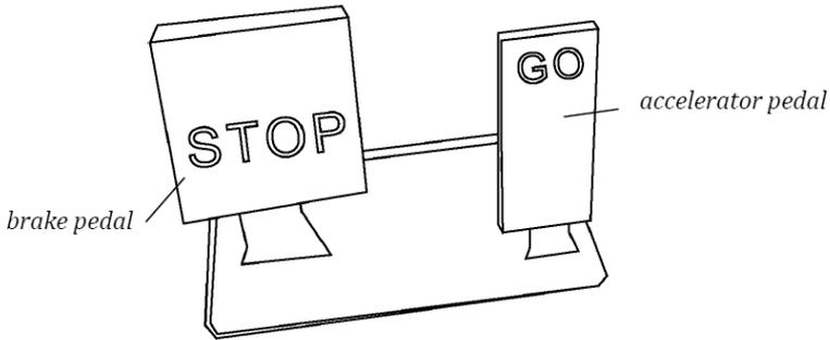
**Accelerator Pedal:** The accelerator pedal can be found on the right side labeled GO. This pedal is different from the accelerator pedal in common car. Turn on the main switch and select the F/R switch to move forward or in reverse and the golf car's speed will accelerate gradually as the accelerator pedal is depressed. Releasing the pedal causes the power to be cut and the motor to stop working gradually.
